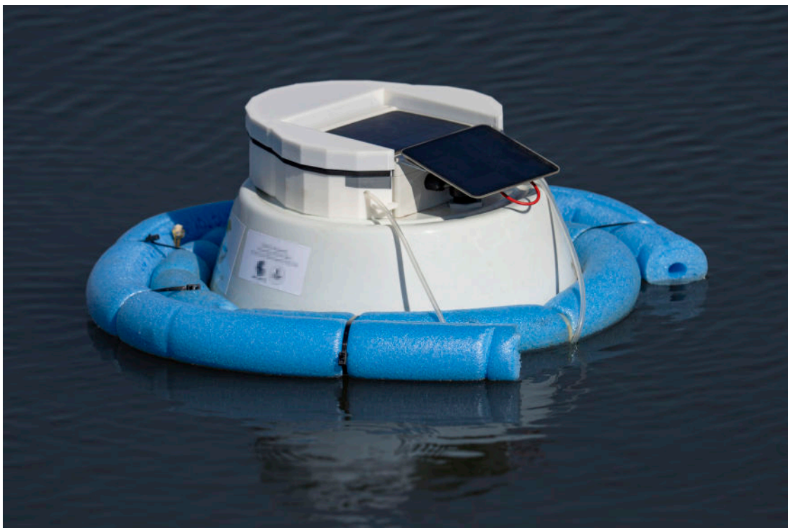
Fig. 3: Photo of a Pondi – one of CNPS' floating greenhouse gas sensors equipped with CO 2 , CH 4 , and N 2 O sensors to continuously measure gas concentrations within the chamber. All data is sent to a cloud via 4G, allowing for the real-time monitor of greenhouse gas fluxes. Each Pondi is equipped with a solar panel for continuous battery charging and a robotic pump (white U-shaped structure) for periodic venting to prevent gas saturation within the chamber.
