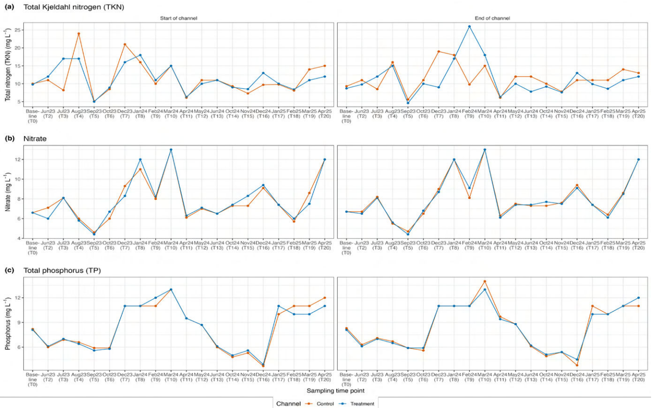
Fig. 6: (a) Total Kjeldahl nitrogen, (b) nitrate, and (c) total phosphorus (in mg L -1 ) at the different sampling locations (start or end of channel) within the control (orange) and treatment (blue) channels across the sampling period.
