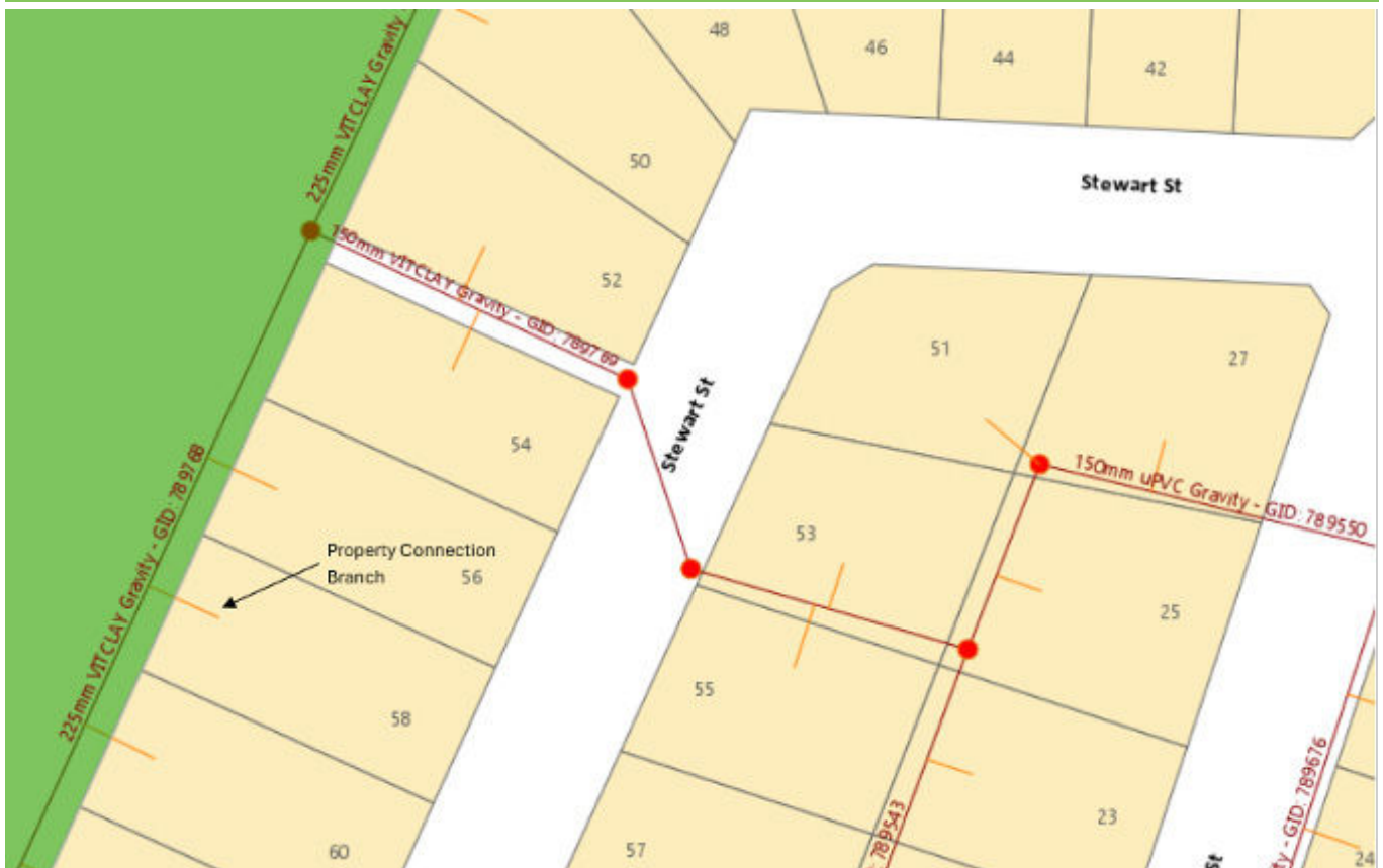
Figure 10: Sewer connection branch-asset plan
